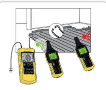
Fault detection in under-floor heating systems
