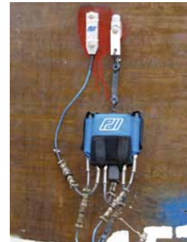
Smart accelerometer and strain transducer, offshore version.
